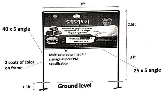
The angle used shall be of Tata/ Jindal make , the structure shall be installed with cement grouting for long life. The boards shall be riveted on the frame.
